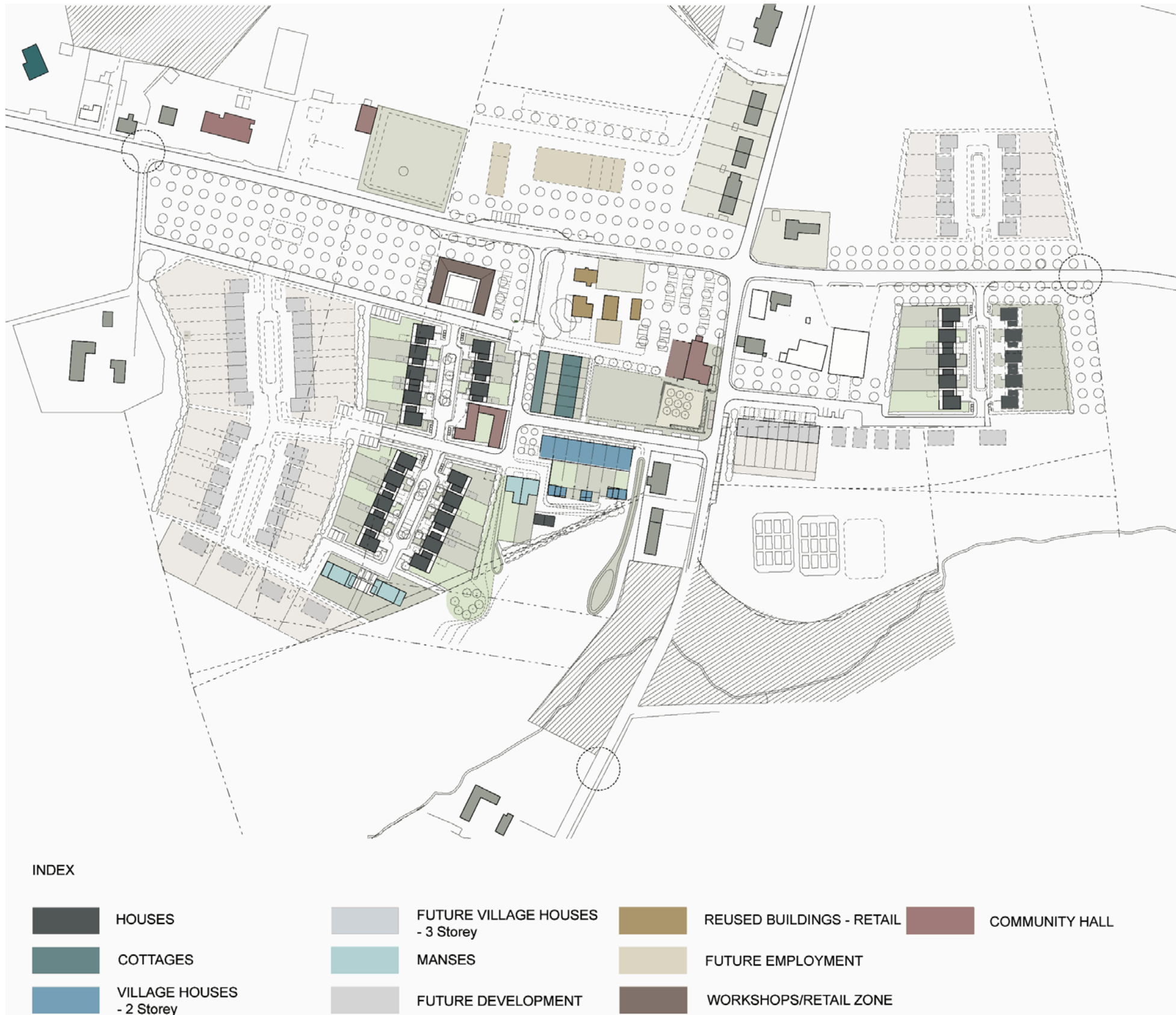
Fig 6.0 Site distribution of building types
