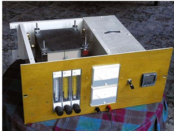
19inch rack mounted fuel cell courtesy of Fuel Cells (Scotland) Ltd
