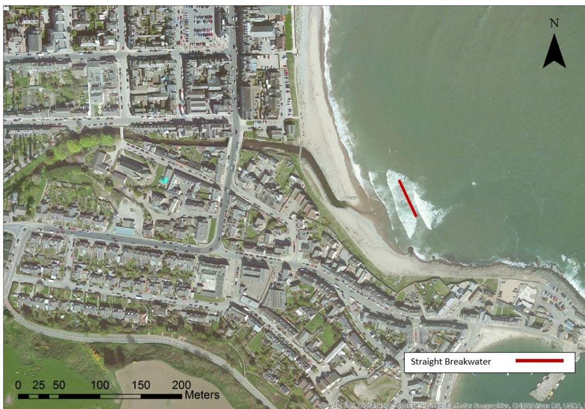
Figure 5-2: Option 2 - Nearshore breakwater.
