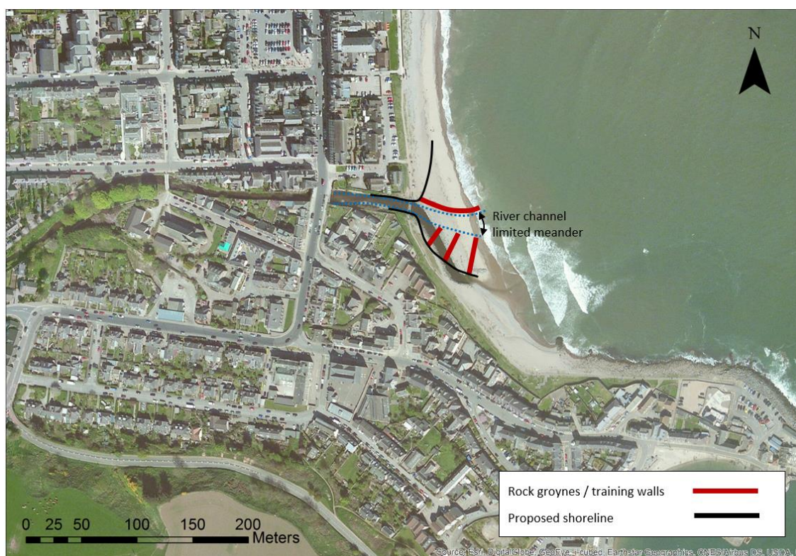
Figure 5-1: Option 1 - Northern training wall and southern groynes.
